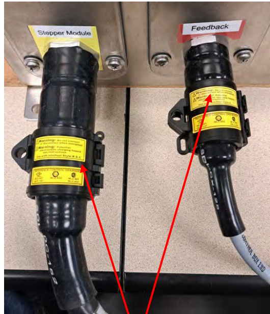
Figure 4D – LockFast secured
