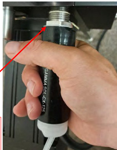
Figure 3B – Small Tubing Position as shrinking begins
