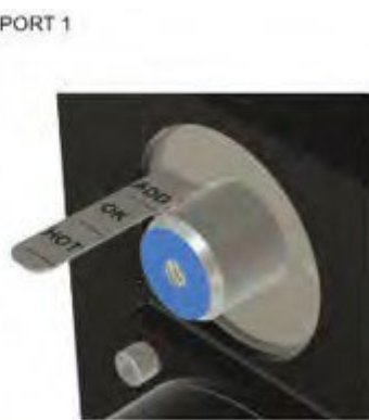
Figure 20: Oil Level Indicator "OK"
