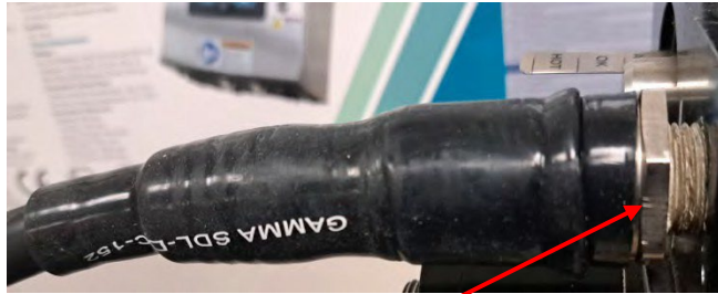
Figure 2B – Large Tubing after shrinking
