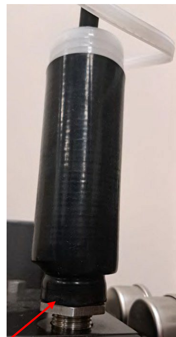
Figure 2A – Large Tubing Position as shrinking begins
