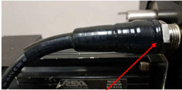
Figure 3C – Small Tubing after shrinking
