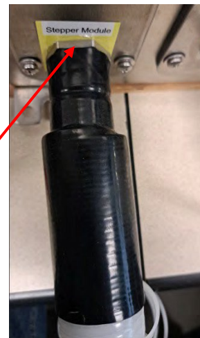
Figure 4B – Tubing Position as shrinking begins
