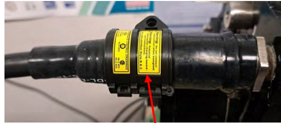
Figure 2C – LockFast secured (Large)
