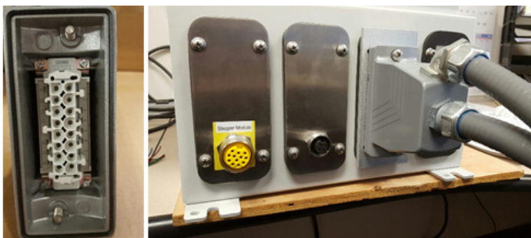
Figure 1.8.4-5 Wire Termination Hub
