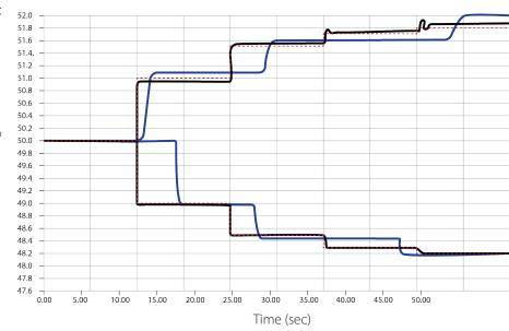
The "Sensitivity Test" performs a series of four increasingly smaller steps in an upward direction, then returns to the offset value and performs the same steps in a downward direction.
