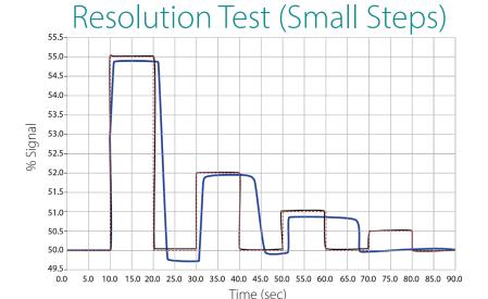
The "Resolution Test" performs four increasingly smaller steps and plots how well the valve responds to each step. For critical control valve applications, the small steps are where **money is made or lost!** Therefore, it's crucial to be able to respond to these small step changes with speed, accuracy, and precision.
