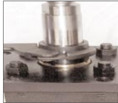
Fig A2: Parker tool for gland removal and installation. (step A.5, A.24)
