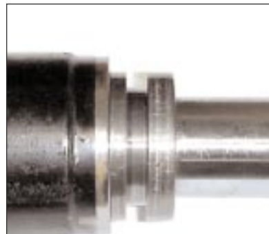
Fig A9: Piston disk ready for second set of seals (step A.16)
