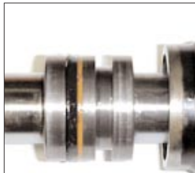
Fig A8: Piston disk with one set of seals into cylinder (step A.15)
