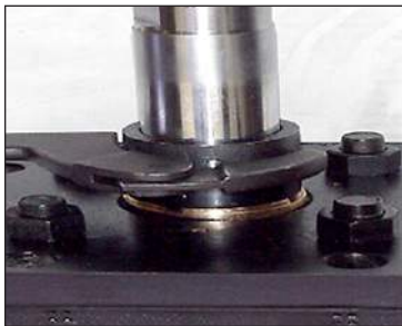
Photo 4M.17.1-3: Parker tool for gland removal
