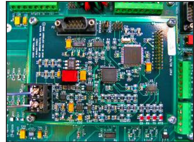
Photo 4.E.13.1-1 HART interface assembly
