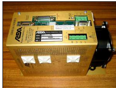
Photo 4.E.9-1 Servo Motor Driver
