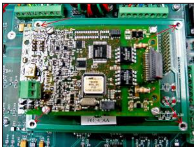
Photo 4.E.14.2-3 Threaded standoff holes
