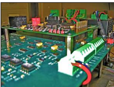
Photo 4.E.13.2-2 Hart board on standoffs
