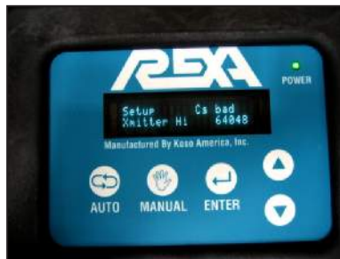
Photo 3.15.4-4 Xmitter Hi readout
