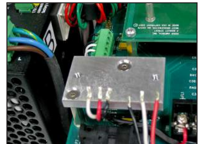
Photo 4.E.16.1-4 Feedback mounting plate
