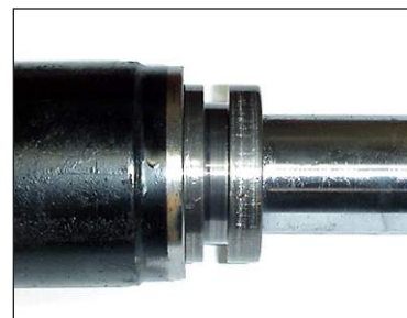
Photo 4M.17.1-9: Piston disk ready for second set of seals
