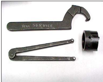
Photo 4M.17.1-2: Tools for gland removal and installation
