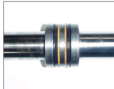
Photo 4M.17.1-7: Piston Disk Assembly
