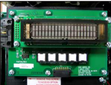
Photo 4.E.11-2 Internal Display Interface
