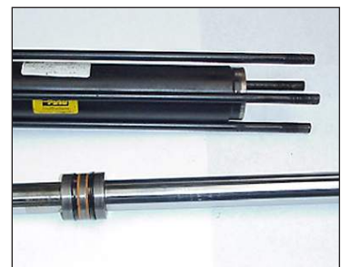
Photo 4M.17.1-5: Piston Rod Assembly
