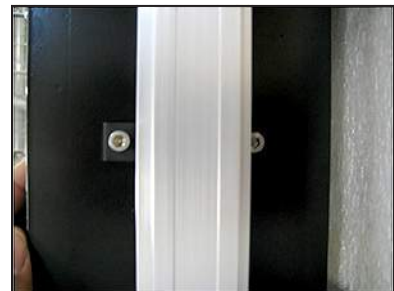
Photo 4.M.21.3-5 Sensor track & mounts
