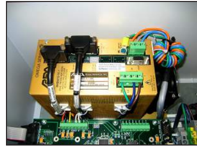
Photo 4.E.9.2-2 Servo Motor Drive Connections
