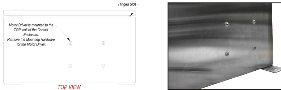
Figure 4.E.11.4-1 Mounting Screw Placement
