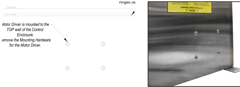
Figure 4.E.10.2-1 Mounting Screw Placement
