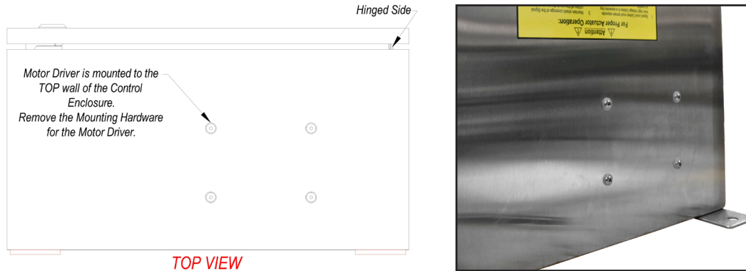
Figure 4.E.9.1-2 Mounting Screw Location
