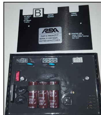
Photo 3.2.1-3 Stepper Driver, Potted Version for Hazloc Shown
