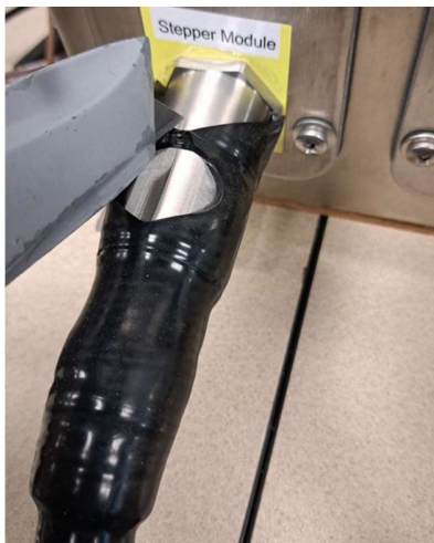
Figure 5A – Remove shrink only from metal nut so cordset can be un-mated from receptacle
